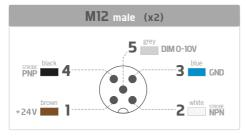
**EMC IMMUNITY CONNECTIONS:** for greater EMC immunity when using the light under Strobe operation, configure the signal connections as illustrated here. For Dimming, the Pin (5) should be connected to a voltage between OV and 10V to ensure light output is correctly configured.
