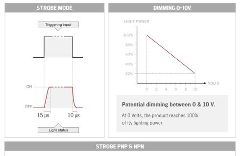
**PNP :** from 5 to 24V for 100% ON. From 0 to 1V for 100% OFF.
