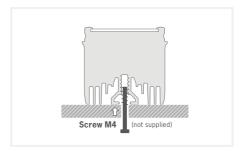
You can also use M4 screws (not supplied) fastened directly into Aluminium profile with a tightening torque from 0.5 to 1.5Nm. We also recommend the use of a threadlocker (not supplied) to avoid any risk of loosening.
