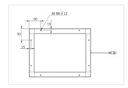
During the set up, the light has to be switched off and unplugged. Please use the fixing holes designed for that purpose (see scheme above). We recommend the using of M6 screws (not supplied) with a tightening torque from 0.5 to 1.5 Nm. We also recommend the use of a threadlocker (not supplied) to avoid any risk of loosening.
