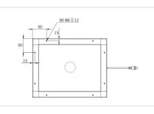
During the set up, the light has to be switched off and unplugged. Please use the fixing holes designed for that purpose (see scheme above). We recommend the using of M6 screws (not supplied) with a tightening torque from 0.5 to 1.5 Nm. We also recommend the use of a threadlocker (not supplied) to avoid any risk of loosening.
