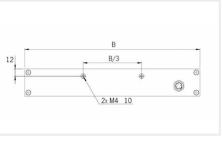
During the set up, the light has to be switched off and unplugged. Please use the fixing holes designed for that purpose (see scheme above). We recommend the using of M4 screws (not supplied) with a tightening torque from 0.5 to 1.5 Nm. We also recommend the use of a threadlocker (not supplied) to avoid any risk of loosening.
