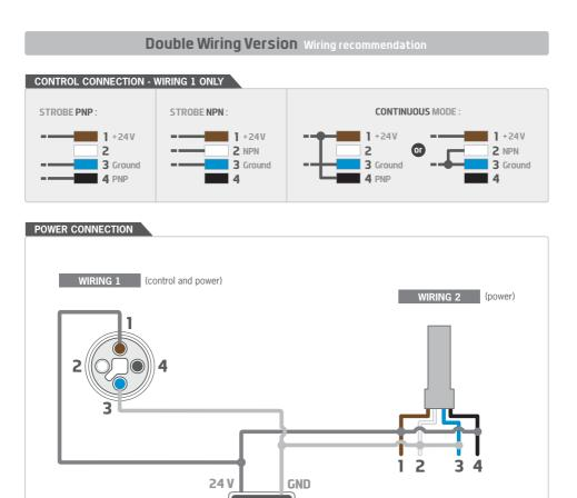
In the **DOUBLE WIRING** version, both wirings can be powered by **THE SAME POWER SUPPLY 24V**.
