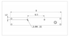
During the set up, the light has to be switched off and unplugged. Please use the fixing holes designed for that purpose (see scheme above). We recommend the using of M4 screws (not supplied) with a tightening torgue from 0.5 to 1.5 Nm. We also recommend the use of a threadlocker (not supplied) to avoid any risk of loosening.
