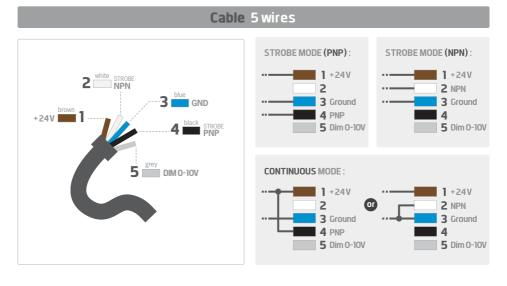
**EMC IMMUNITY CONNECTIONS:** for greater EMC immunity when using the light under Strobe operation, configure the signal connections as illustrated here. For Dimming, the Pin (5) should be connected to a voltage between 0V and 10V to ensure light output is correctly configured.
