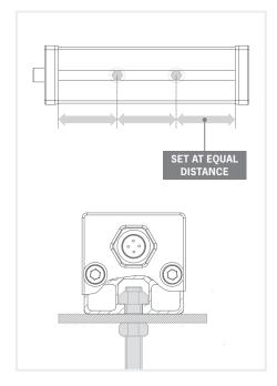
During the set up, the light has to be switched off and unplugged. Please use the 2 delivered nuts and insert them in the groove located in the back of the lighting. The lighting will be better fixed if you spread the attachment points as indicated on the scheme above.
