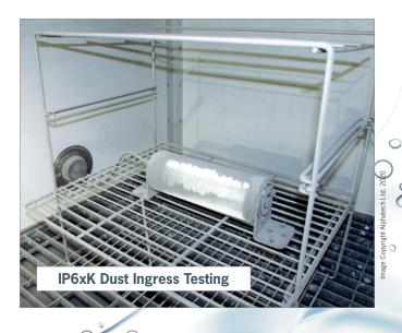
TPL Vision's Washdown Lights also go through a rigorous IP69K certification process to confirm that the light can withstand the cleaning process and continue to operate, without moisture or particle ingress, meaning you can have complete confidence in using them in your washdown environment.
