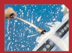
Operating LED lights within Food or Pharmaceutical manufacturing processes with regular sanitising / washdown operation requires an **IP69K** rated package. Operating across wide temperature ranges, high humidity environments, and cleaning with hot or cold cleaning agents produces a significant design challenge for the LED **Illumination manufacturer**. It's not as simple as just mounting a light within a fluid tight box.
