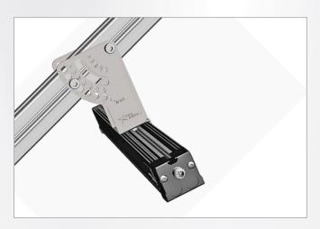
The **Bar BMOUNT** is a clever mount, that enables the easy setting of TPL Vision's LED bars in machine vision systems. Thanks to the **Bar BMOUNT**, you can adjust the angle of incidence precisely (from 0° to 60°), using the dedicated holes (1 hole every 10°).
