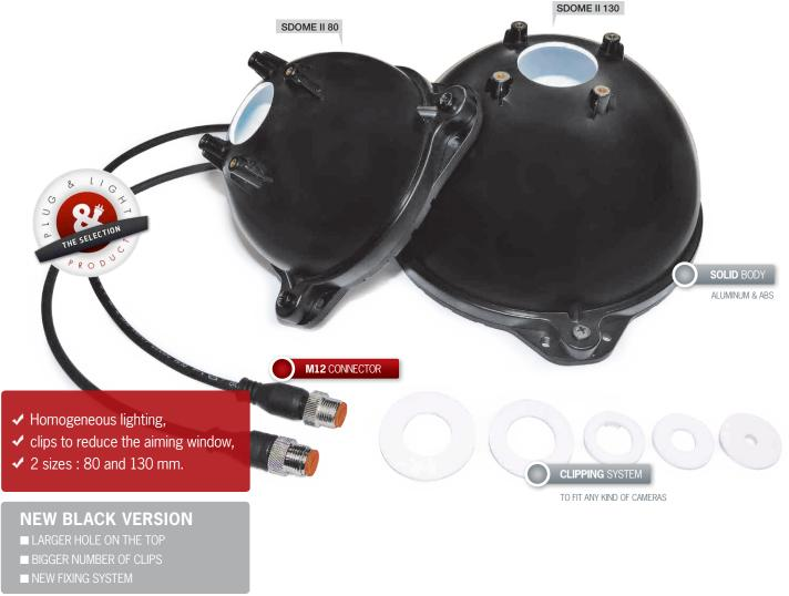
Equipped with new leds, the SMALL SDOME II gets a lighting power 4 to 5 times higher than the previous version used to have for white and red leds (WHI & 630). The SMALL SDOME II offers a diffuse and homogeneous indirect lighting that lessen reflections and enable a reliable quality control process on curved and shiny surfaces. This is the ideal lighting for bar codes and 2D codes reading. Thanks to
