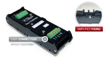
The **Time TCONTROL** is an electronics module that enables the control and the regulation of current in TPL Vision's led lightings manufactured without electronics (SE), only in strobe mode. Thanks to the **Time TCONTROL**, you can supply the lighting with power, regulate the current, control the rising time and control the camera triggering (from 5 ms to 1 000 ms).
