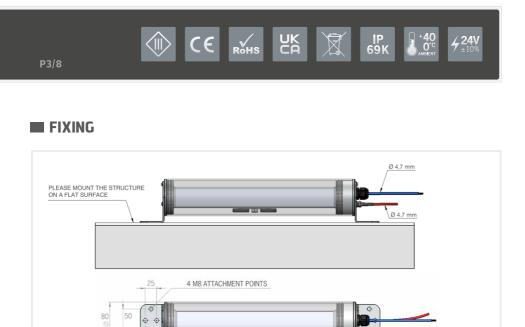
**BEWARE:** if you don't want to use the brackets supplied with the product on a flat surface, here are our recommendations. **1** - You can use clamps. Please place them on the o-ring of the tube. Do not press it, to avoid any pressure or fissure.
