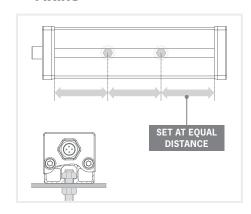
During the set up, the light has to be switched off and unplugged. Please use the 2 delivered nuts and insert them in the groove located in the back of the lighting. The lighting will be better fixed if you spread the attachment points as indicated on the scheme above.
