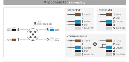
**PNP :** from 5 to 24V for 100% ON. From 0 to 1V for 100% OFF. **NPN :** less than 1V for 100% ON. Above 2V for 100% OFF. Max 20V.
