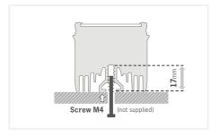
You can also use M4 screws (not supplied) fastened directly into Aluminium profile with a tightening torque from 0.5 to 1.5Nm. We also recommend the use of a threadlocker (not supplied) to avoid any risk of loosening.
