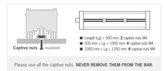
During the set up, the light has to be switched off and unplugged. Please use M4 screws and insert them in the captive nuts located in the back of the light. The light will be better fixed if you spread the attachment points symmetrically along the bar.
