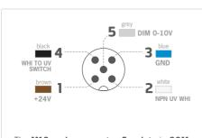
The **M12** male connector **5** points is **COM-PLIANT** with the M12 female connector 4 points. In that case, the dimming option is not available.
