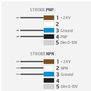
**PNP** : from 5 to 24V for 100% ON. From 0 to 1V for 100% OFF.
