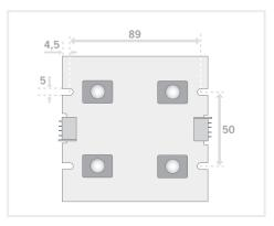
During the set up, the light has to be switched off and unplugged. Please use the fixing holes designed for that purpose (see scheme below). We recommend the using of M4 screws (not supplied) with a tightening torque from 0.5 to 1.5 Nm. We also recommend the use of a threadlocker (not supplied) to avoid any risk of loosening.
