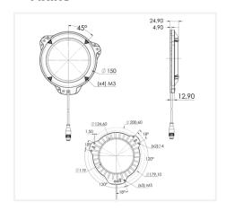
During the set up, the light has to be switched off and unplugged. Please use the fixing holes designed for that purpose (see scheme above). We recommend the using of M5 screws (not supplied) with a tightening torque from 0.5 to 1.5 Nm. We also recommend the use of a threadlocker (not supplied) to avoid any risk of loosening.
