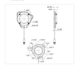
During the set up, the light has to be switched off and unplugged. Please use the fixing holes designed for that purpose (see scheme above). We recommend the using of M5 screws (not supplied) with a tightening torque from 0.5 to 1.5 Nm. We also recommend the use of a threadlocker (not supplied) to avoid any risk of loosening.
