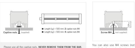
During the set up, the light has to be switched off and unplugged. Please use M4 screws and insert them in the captive nuts located in the back of the light. The light will be better fixed if you spread the attachment points symmetrically along the bar. You can also use M4 screws (not supplied) fastened directly into Aluminium profile with a tightening torque from 0.5 to 1.5 Nm. We also recommend the use of a threadlocker (not supplied) to avoid any risk of loosening.
