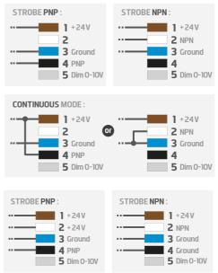
**EMC IMMUNITY CONNECTIONS:** for greater EMC immunity when using the light under Strobe operation, configure the signal connections as illustrated here. For Dimming, the Pin (5) should be connected to a voltage between OV and 10V to ensure light output is correctly configured.
