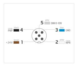
EMC IMMUNITY CONNECTIONS: for greater EMC immunity when using the light under Strobe operation, configure the signal connections as illustrated here. For Dimming, the Pin (5) should be connected to a voltage between OV and 10V to ensure light output is correctly configured.
