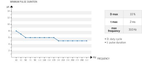
Don't exceed 310 Hz when strobing PNP/NPN in overdrive mode.
