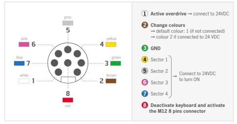
REMOTE CONTROL PINOUT THROUGH PNP: 0-4V is OFF and 5-24V is ON.
