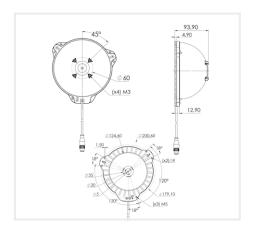
During the set up, the light has to be switched off and unplugged. Please use the fixing holes designed for that purpose (see scheme above). We recommend the using of M5 screws (not supplied) with a tightening torque from 0.5 to 1.5 Nm. We also recommend the use of a threadlocker (not supplied) to avoid any risk of loosening.
