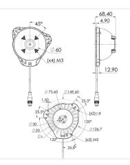
During the set up, the light has to be switched off and unplugged. Please use the fixing holes designed for that purpose (see scheme above). We recommend the using of M5 screws (not supplied) with a tightening torque from 0.5 to 1.5 Nm. We also recommend the use of a threadlocker (not supplied) to avoid any risk of loosening.
