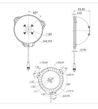
During the set up, the light has to be switched off and unplugged. Please use the fixing holes designed for that purpose (see scheme above). We recommend the using of M5 screws (not supplied) with a tightening torque from 0.5 to 1.5 Nm. We also recommend the use of a threadlocker (not supplied) to avoid any risk of loosening.
