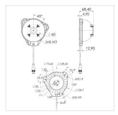
During the set up, the light has to be switched off and unplugged. Please use the fixing holes designed for that purpose (see scheme above). We recommend the using of M5 screws (not supplied) with a tightening torque from 0.5 to 1.5 Nm. We also recommend the use of a threadlocker (not supplied) to avoid any risk of loosening.
