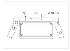
During the set up, the light has to be switched off and unplugged. Please use the fixing holes designed for that purpose (see scheme above). We recommend the using of M3 screws (not supplied) with a tightening torque from 0.5 to 1.5 Nm. We also recommend the use of a threadlocker (not supplied) to avoid any risk of loosening.
