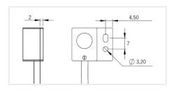
During the set up, the light has to be switched off and unplugged. Please use the fixing holes designed for that purpose (see scheme above). We recommend the using of M3 screws (not supplied) with a tightening torque from 0.5 to 1.5 Nm. We also recommend the use of a threadlocker (not supplied) to avoid any risk of loosening.
