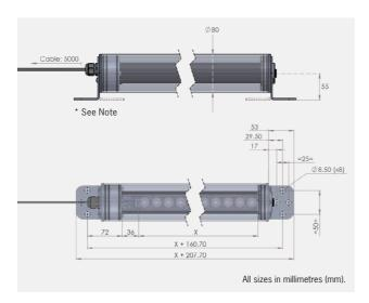
NOTE: the Swivel L-Brackets (360 Degrees) illustrated (\*) are included with the product. The brackets are designed with dual mounting orientations, allowing them to be positioned with the flange either outward from the product or tucked beneath it.
