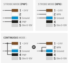
**EMC IMMUNITY CONNECTIONS:** for greater EMC immunity when using the light under Strobe operation, configure the signal connections as illustrated here. For Dimming, the Pin (5) should be connected to a voltage between 0V and 10V to ensure light output is correctly configured.
